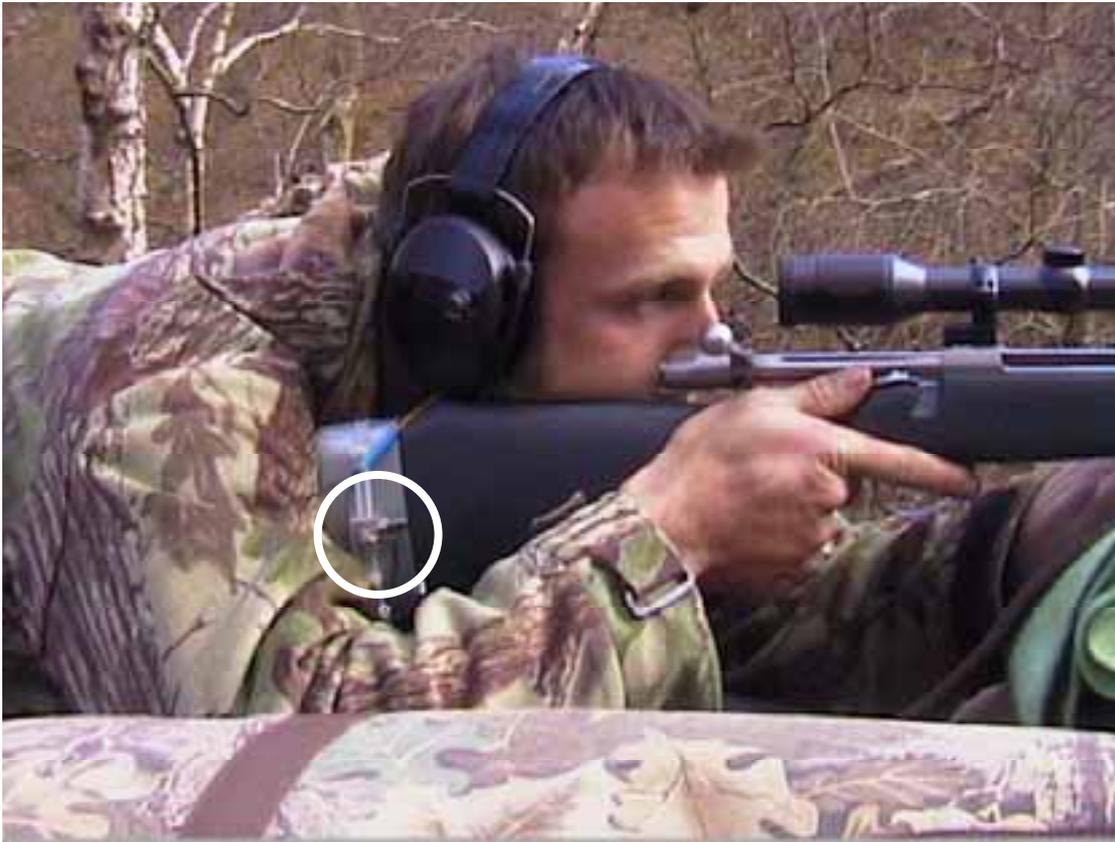
**Figure 3 Accelerometers fitted on stock**
